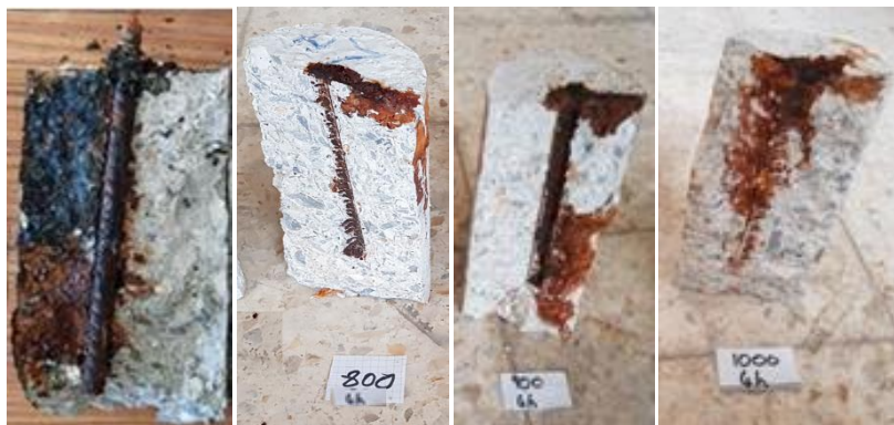
Figure 6. Inner view of corroded Ø14 reinforced samples depending on boriding temperature
