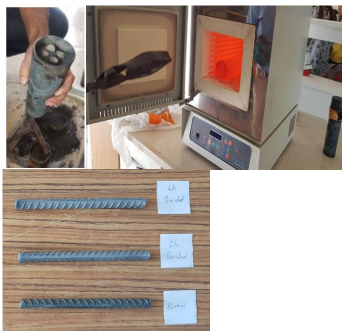
Figure 1. Coating process of rebar by boriding
