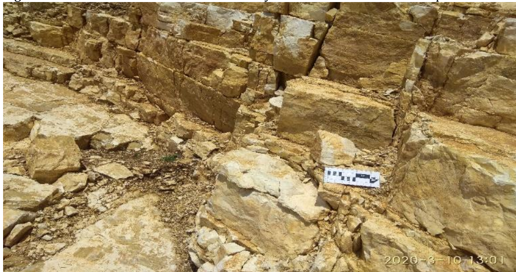
Figure 20. Orientation of the main joint sets.
