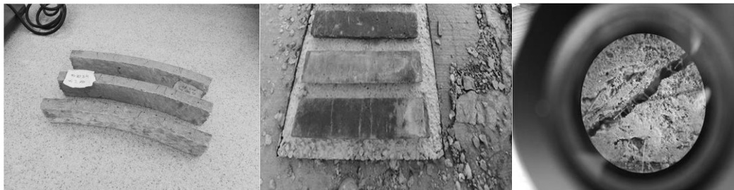
Figure 2. Small mortar beams for self-healing measurement
