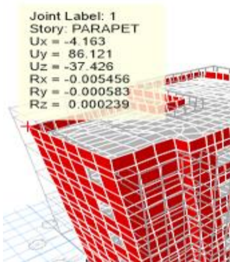
Fig. 3 – Displacements for the original building
