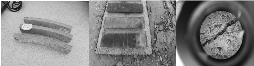
Figure 2. Small mortar beams for self-healing measurement
