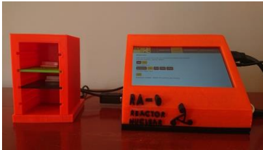
Figure 8: Simulated absorption experiment setup
