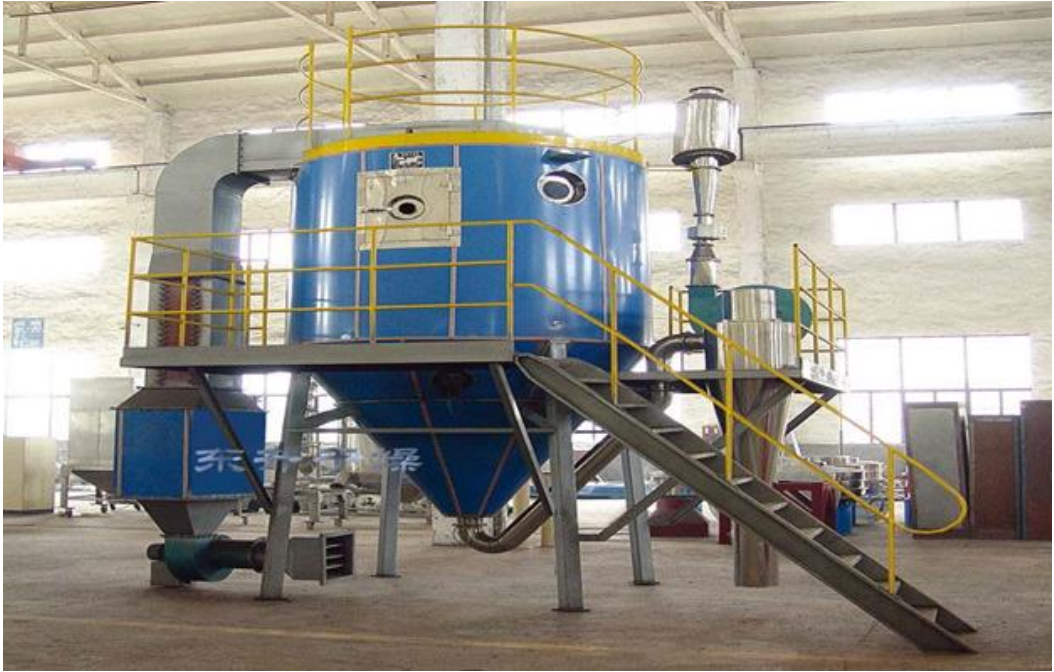
Fig. 3. Industrial spray dryer
