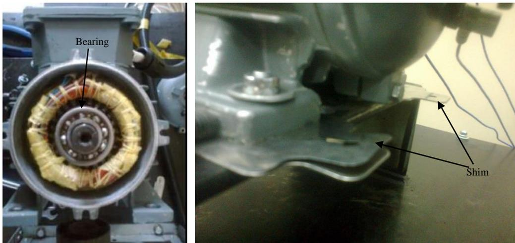
a) Tested bearing lubricated
