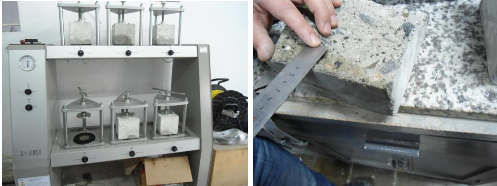
Figure 3.2.1: Images of water penetration
